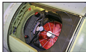
The German-built 100-inch telescope that is the heart of NASA's Stratospheric Observatory for Infrared Astronomy is nestled in the SOFIA 747's rear fuselage. (Photo courtesy of L-3 Communications)
